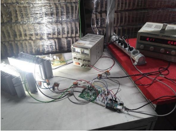
Fig. 4. Test bench with all parts mounted for the MPPT testing.
